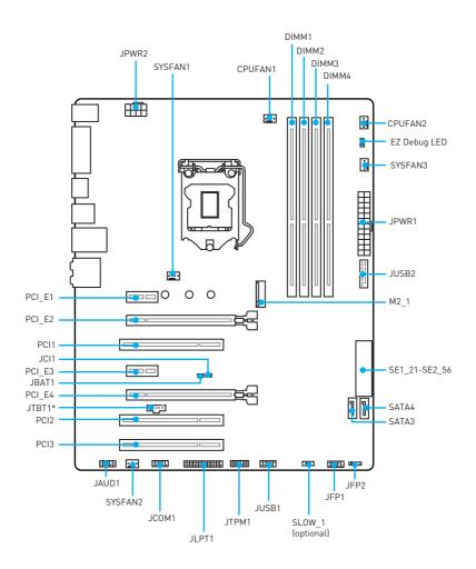
Note: The JTBT1 connector and the PCI\_E4 slot can't be used simultaneously.
