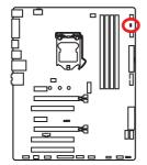
**□ VGA** - indicates GPU is not detected or fail. **DRAM** - indicates DRAM is not detected or fail. **CPU** - indicates CPU is not detected or fail.
